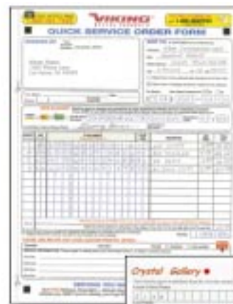
Traditional TELEform Form Fixed cornerstones and form ID code make traditional TELEform forms ideal for fax-based applications.
